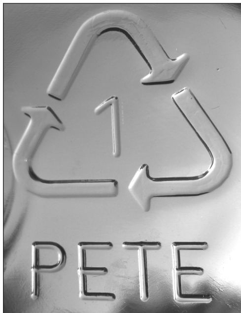
Figure 1. Close-up of a container made using PETE with a recycle code of 1. (Photo credit: Hal Harris.)
